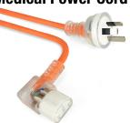
A 3-core general duty power cord fitted with a left-hand right-angle IEC-C13 connector and Australian 3-pin mains plug with insulated pins compliant with AS/NZS3112. Orange coloured flex and transparent mains plug & IEC connector as required for medical equipment applications. Electrical Safety Authority Approved.
