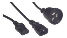
10 Amp 3-core power cord fitted with one IEC-C14 connector, one IEC-C13 connector and one 3-pin Australian mains socket. Suitable for connection of a device fitted with a standard Australian mains plug and a device fitted with an IEC-C14 connector to a UPS or other device fitted with a IEC-C13 female connector. Length is 600mm overall, comprising 2 x 220mm IEC sections and a single 220mm section from the mains socket to the Y-junction. Electrical Safety Authority Approved.
