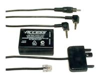
Compact LIU allows any audio device having an earphone or line-out socket to be connected to any compatible Key Telephone or PABX system to provide music to calls that are placed on hold. Incorporates a recessed potentiometer to adjust volume level. The Source cords are 600mm long. The length of the System cord is shown in the table below.
