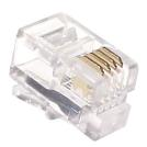
Generally used for termination of coiled handset cords. Plugs with  $50\mu^n$ ,  $30\mu^n$  or  $15\mu^n$  gold plated contacts are available. Packed in bags of 5, 20, 50, 100 or bulk. Plugs for stranded or solid conductors with round or flat cord entry are available.
