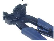
Precision hand crimp employs a ratchet action ensuring correct crimping pressure is applied for reliable, trouble-free compression of our P0720 series water-proof BNC, RCA, PAL and F-type coax connectors. Adjustable compression depth.
