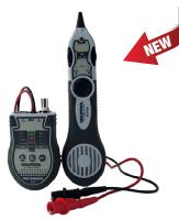
Wiring system tester, connection map test for discontinuity, short circuit, reversed pairs, crossed pairs, wire tracing, cable continuity, polarity and verifying a line. Possibility of identifying & tracing wires or cables with no damage to insulation. Max.1km cable length, min. receiver distance: 60cm. Signal frequency 500-781Hz, signal frequency 500Hz~781Hz
