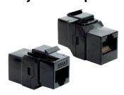
Cat6 coupler for use with Keystone patch panels, and flush plates. Allows ready-made Cat6 patch cords to be used in fixed installations eliminating the use of IDC terminations and tools. Can also be fitted to Australian HPM and Clipsal flush plates by using Clipsal and HPM keystone bezels (DATAMASTER P4590 Clipsal and P4592 HPM) The 1-1 wiring configuration is compatible with both T568A and T568B wiring schemes. Colour is black.
