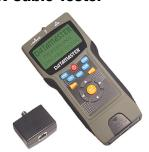
Professional LAN cable tester with advanced backlit LCD. Tests and displays exact pin-to-pin wiring configuration of LAN cables, modular telephone cables and coaxial cables. Tests and displays length of LAN or coaxial cables. With remote terminator (ID #01) for near-end/far-end testing of installed network cables on site, 2 x F-type to BNC coax adaptors, 2 x 8P to 6P modular reducers and 9V battery.
