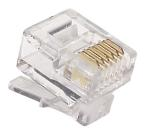
6 position MMP (also known as MMJ or DEC-connect) type with offset latch as used for specific computer systems. Plugs with  $50\mu^{\rm m}$  or  $30\mu^{\rm m}$  gold plated contacts are available. Packed in bags of 20, 50, 100 or 1000. Plugs for stranded or solid conductors with round or flat cord entry are available.
