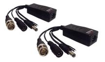
Used to carry CCTV video signal, power feed and data for PTZ over Cat5e or Cat6 cable. Passive design transmits colour video up to 400 metres, 12V or 24V, power feed up to 250 metres and PTZ data up to 300 metres. Integrated surge protection. Male BNC for video connections, male/female barrel plug/socket for power feed, RJ45 modular socket for connection to the Cat5e or Cat6 cable and tinned ends for PTZ data connection. Packed in a blister pack set of two.
