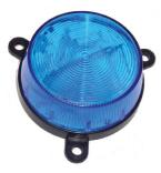
This 12 volt, 3 watt strobe light is suitable for connection to our Universal Loud Sounding Alarm or for use with alarm systems, indicator-boards etc. Three lugs allow mounting to any surface. Two 550mm conductors exit from the centre rear of the unit and have tinned ends for easy termination.
