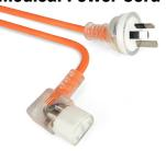
A 3-core general duty power cord fitted with a left-hand right-angle IEC-C13 connector and Australian 3-pin mains plug with insulated pins compliant with AS/NZS3112. Orange coloured flex and transparent mains plug & IEC connector as required for medical equipment applications. Electrical Safety Authority Approved.
