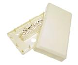
Ivory coloured surface-mount distribution box with cable entry holes in rear and cable entry cut-outs on all 4 sides. Contains a 10-pair IDC module constructed of high-impact fire-resistant PBT material with corrosion resistant 5.0 micron silver-plated terminals. Terminate wires using our T0059 impact tool (or any impact tool designed for termination of Krone-type IDC terminals). Supports pair-disconnect function if appropriate test plug is inserted. Dimensions 164(H) x 85(W) x 36(D)mm.
