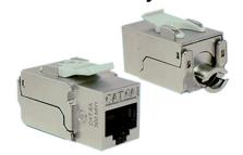
Suitable for use with all Keystone flush plates, surface boxes and Cat-6A shielded keystone patch panels including our DATAMASTER range. Can also be fitted to Australian HPM and Clipsal flush plates by using Clipsal and HPM keystone bezels. (DATAMASTER P4590 Clipsal and P4592 HPM) Terminated with 110 IDC Impact Tool. Combined T568A & T568B colour coding for easy installation. Packaged in individual bags.
