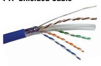
FTP (Foil Twisted Pair) Cat6 cable for premises wiring and applications where shielded cable is required. 4 twisted pairs with solid copper conductors suitable for IDC terminations to patch panels and wall jacks. Conductors are wrapped with aluminium foil shield and Mylar tape. Tinned drain wire. Available on durable 305 metre reels. Count-down metre-marking.
