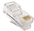
Similar to the standard 6 position modular plug but has a long body as required to mate with deeply recessed modular sockets. Plugs with  $50\mu$ ",  $30\mu$ " or  $15\mu$ " gold plated contacts are available. Packed in bags of 20, 50, 100 or 1000. Plugs for stranded or solid conductors with round or flat cord entry are available.
