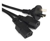
A 10 Amp 3-core power cord fitted with Australian 3-pin mains plug with insulated pins compliant with AS/NZS3112 and two IEC-C13 connectors. Suitable for supply of power to both a PC and monitor from a single power outlet. Length is 2 metres overall, comprising 2 x 1.5 metre IEC-C13 sections and a single 500mm section from the mains plug to the Y-junction. Electrical Safety Authority Approved.
