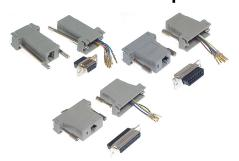
Adapts male or female DB9, DB15 or DB25 connectors plugs to 8 position RJ45 or 6 position RJ11 modular socket. Back shell is pre-wired to modular socket ready to insert pins into desired positions of the DB connector.
